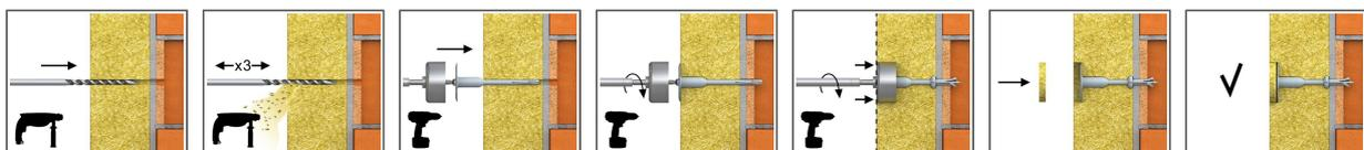
1. [Russian]: Drill a hole of required diameter and depth.
