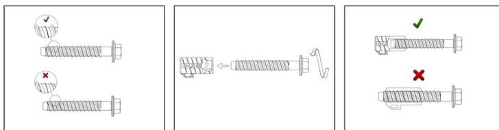
1. [Russian]: Visual assessment. The anchor thread shall not be damaged.
